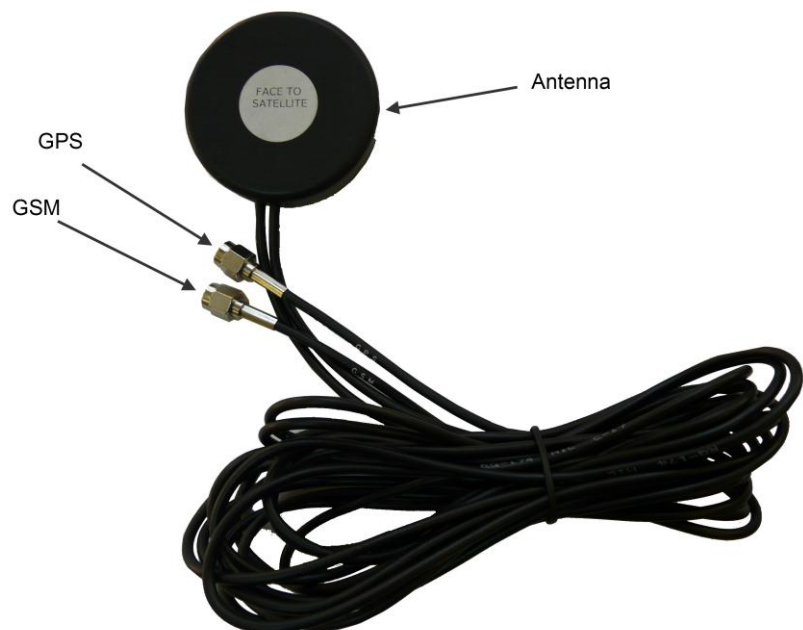
Picture 2 – Connecting antenna to Roadstar
