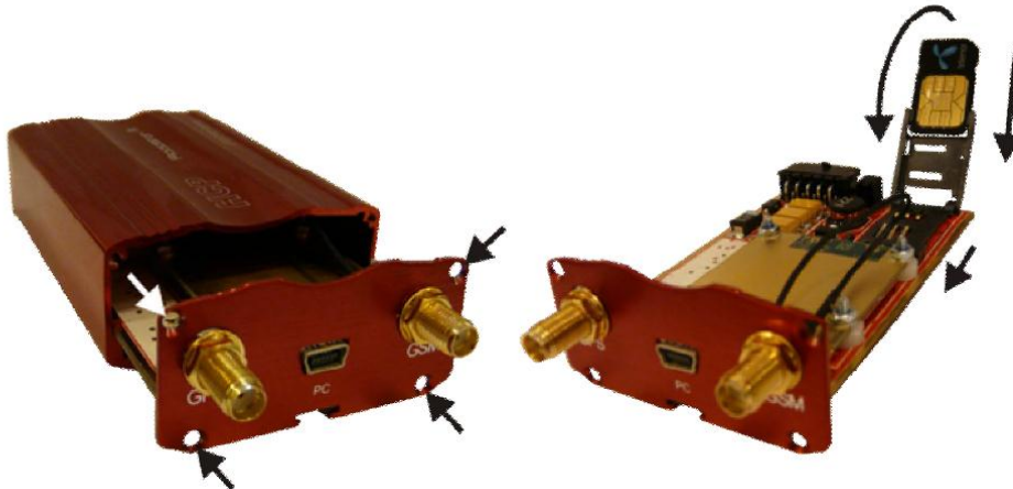
Picture 1 – Placing SIM card
